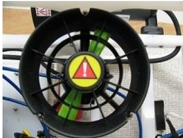
Figure 3-2: Protective thruster shroud.
