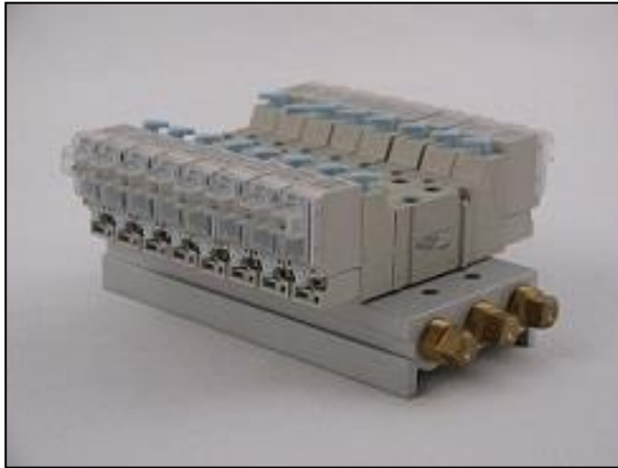
Figure 1-8: The valve bank which supplies all the pneumatic tools.
