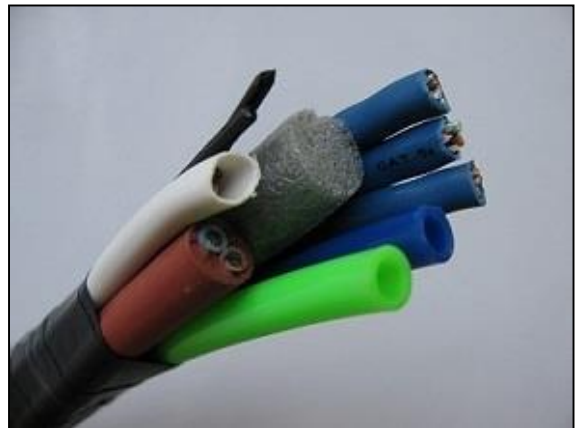
Figure 1-12: A cross section of the complete tether.
