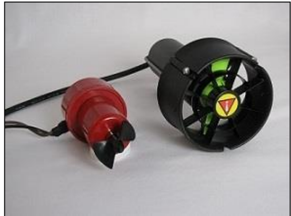
Figure 1-4: Thrusters used for navigation: modified bilge pump on the left, Seabotix thruster on the right.
