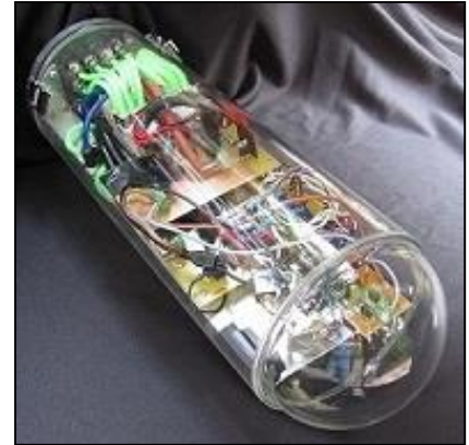
Figure 1-9: The main waterproof canister.
