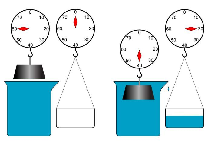
Figure 2: Archimedes Principle – The Buoyant Force is Equal to the Weight of the Displaced Water
