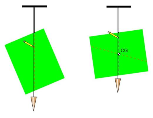
Figure 9: Locating the Center of Gravity Using a Plumb Line
