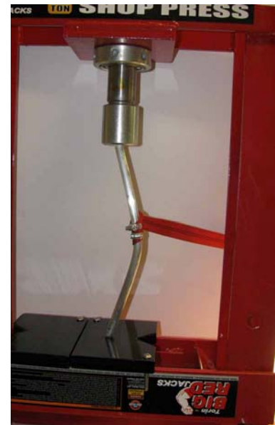
10.7 mm Rod Buckling
