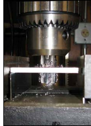
Figure 3: Gland Hole Tapped
