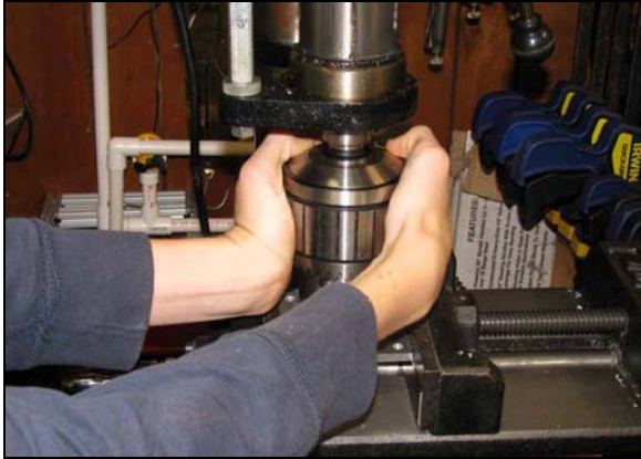
Figure 2: Hand Tapping with a Drill Press
