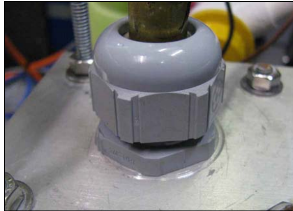
Figure 4: Gland in Canister End Cap
