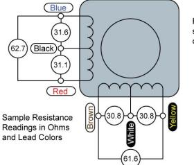
For example, Jameco #155433 stepper motor datasheet shows a resistance/phase (RAB, RBC, RDE, and REF) of 30 Ohms +/- 10%.
