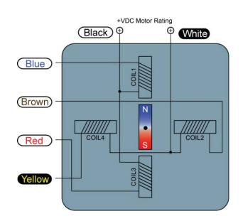
Figure 14: #155433 Stepper Connections to This Point
