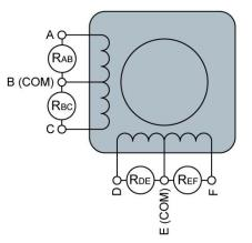
$R_{AB} = R_{BC} = 1/2 R_{AC}$  $R_{DE} = R_{EF} = 1/2 R_{DF}$
