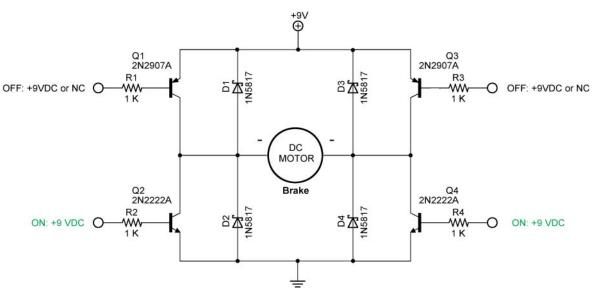
Braking: R2 and R4: +9 VDC with R1 and R3: +9VDC or No Connection
