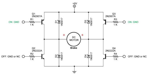
Figure 8: Braking
