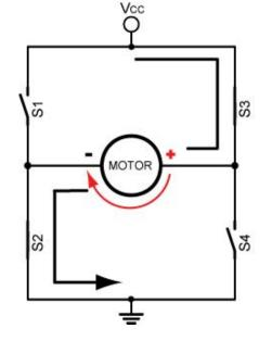
Figure 3: Motor Runs "Forward" (Switches 1 and 4 Closed)
