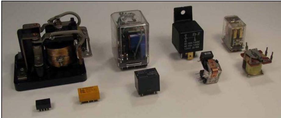
**Figure 1: Assortment of Mechanical Relays**
