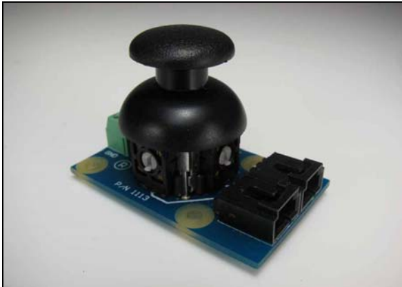
Figure 16: Mini-Joystick with Two Small Potentiometers at Right Angles
