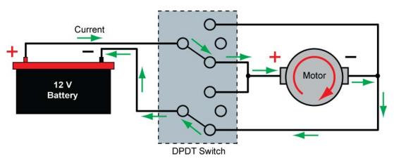
Figure 18: Toggle Down – Clockwise Rotation
