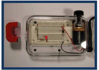
Figure 7: Without any direct mechanical connection with the switch, the magnet closes the reed switch and the LED is illuminated.
