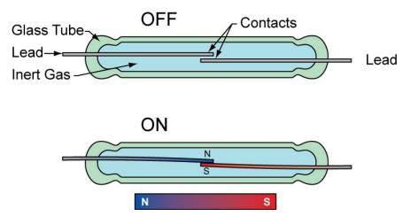
Figure 5: Function of a Reed Switch
