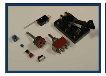
Figure 1: An Assortment of Manual Switches
