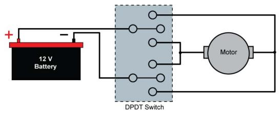
Figure 17: Toggle Center – Motor OFF
