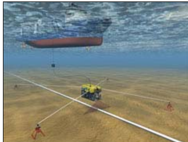
Figure 14: Example of Seabed Grid Acoustic Positioning System
