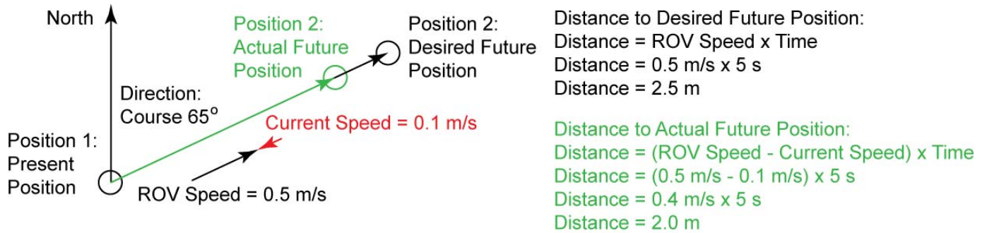
Figure 6: ROV Speed Lowered by Opposing Current
