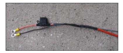
Figure 17: Completed Power Connection
