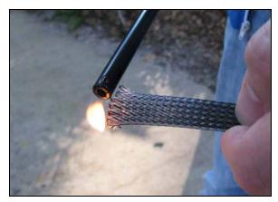
Figure 23: Fuse Filament Ends with Small Flame
