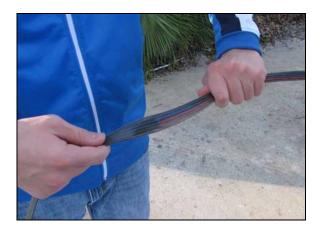
Figure 25: Pushing Sleeving over End
