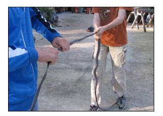
Figure 26: Work the Sleeving Down the Tether
