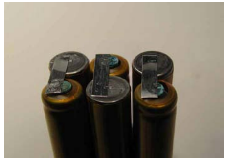
Figure 3: 6 – 1.5 Volt Cells Are Connected in Series to Form a 9 Volt Battery
