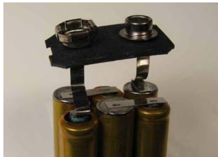
Figure 3: 6 – 1.5 Volt Cells Are Connected in Series to Form a 9 Volt Battery
