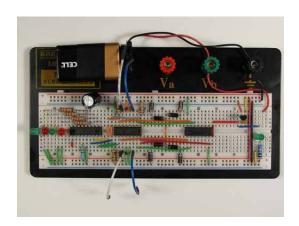
Figure 16: Photo of an H-bridge Circuit
