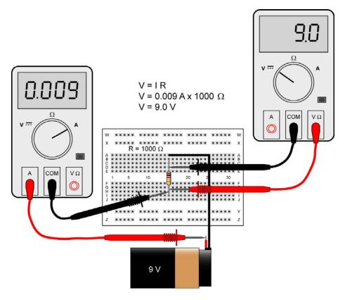
Figure 8: Using a Digital Multimeters to Demonstrate Ohm's Law – Ammeter on Left Is Inserted into the Circuit, the Voltmeter on Right is Parallel to the 1K Resistor See Ohm's Law applets at:
