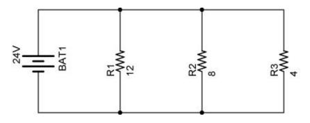
Figure 25: Resistors in Parallel
