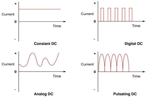
Figure 21: Direct Current Waveforms
