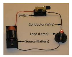
Figure 9: Simple Circuit
