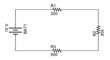
Figure 23: Resistors in Series
