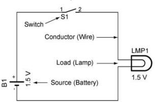
Figure 10: Schematic Diagram of Simple Circuit
