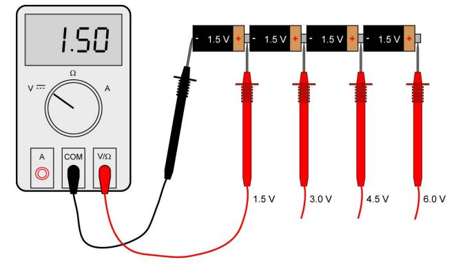
DC voltage sources can also be placed in series to increase the voltage available.
