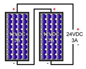
Figure 24: Solar Panels in Series – Voltages Add, Amperage Remains the Same
