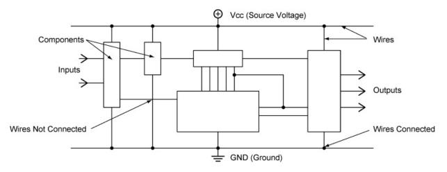
Figure 18: General Layout of a Schematic Drawing
