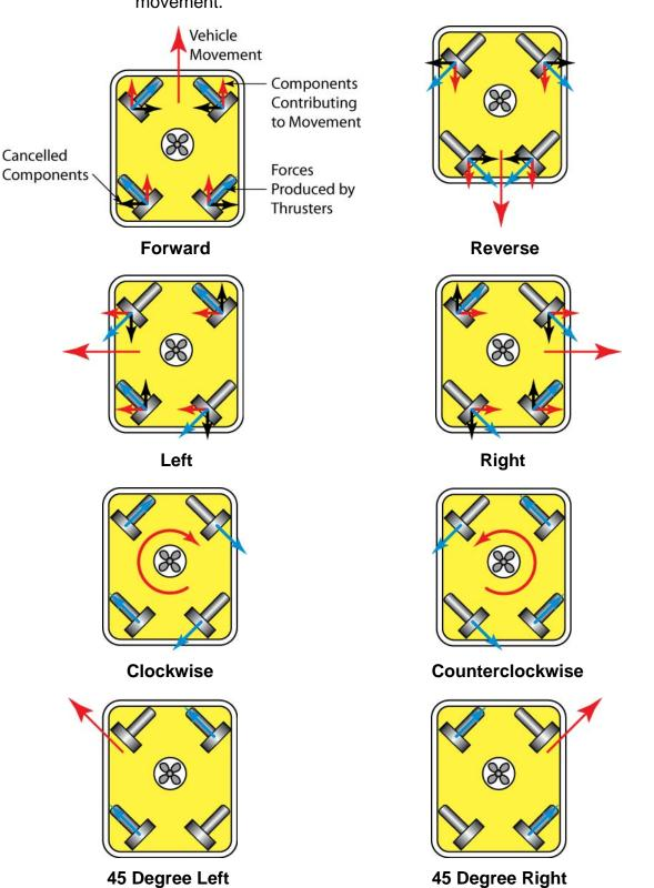
The four horizontal thruster arrangement offers versatility in horizontal movement.
