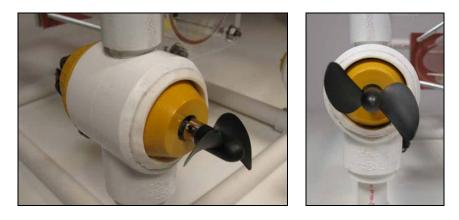
Figure 10: Thruster Mount in Line with Frame Member
