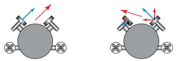
Figure 14: A Couple of Possible Movements if Thrusters Speeds Are Independently Controlled
