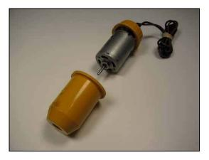
Figure 5: Cutting Too Close to the Motor Breaks the Waterproof Seal
