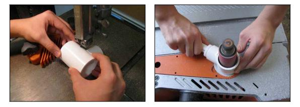
Figure 11: Cutting and Reaming the Reducing Tee
