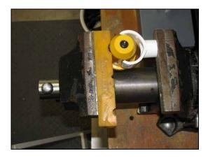
Figure 8: Pressing the Bilge Pump into the Modified PVC Tee
