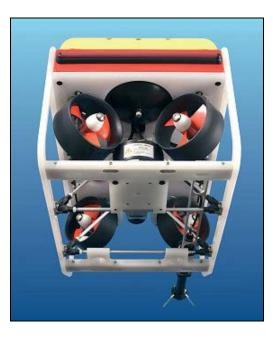
Figure 15: Four Vectored Thrusters for Horizontal Movement From: <u>http://www.seaeye.com/falcon.html</u>
