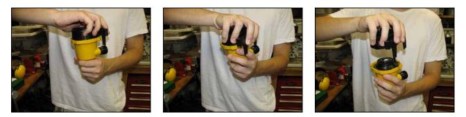
Figure 1: Twist Bilge Pump Unit to Remove
