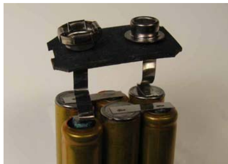
1.5 Volt Cells Are Connected in Series to Form a 9 Volt Battery
