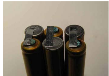
1.5 Volt Cells Are Connected in Series to Form a 9 Volt Battery
