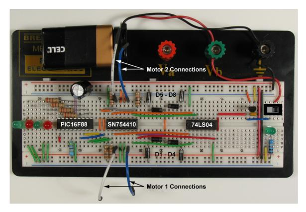
**Breadboard Layout Includes PIC16F88 (Lab 6)**
