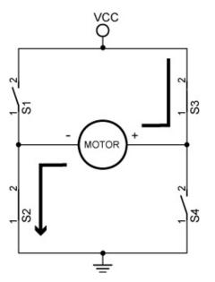
Motor Runs Clockwise (Switches 1 and 4 Closed)
