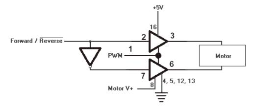
Figure 13: Connections to SN754410
