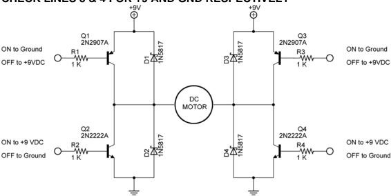
Tie the inputs of Q1 and Q2 together and also connect the inputs of Q3 and Q4 together. What purpose do these connections serve?
