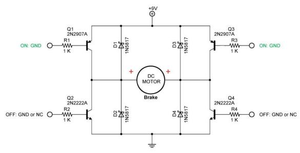
Figure 7: Braking
