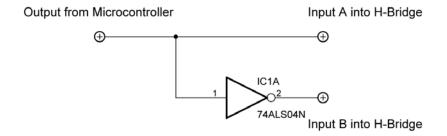
Figure 11: Single Output H-Bridge Driver
