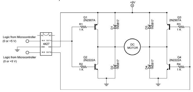
Figure 10: 4427 IC Connection to the H-Bridge
