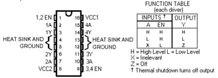
Figure 12: Pinout for the SN754410
