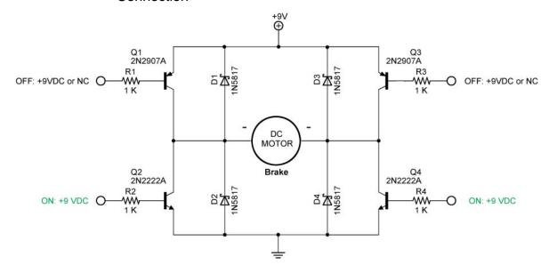
Figure 8: Braking
