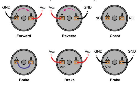
Figure 1: Four States of a DC Motor Output and Their Connections
