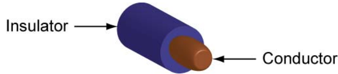
Figure 16: Conductor and Insulator in a Wire
