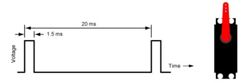
1.5 ms Pulse Width and Corresponding Servo Position
