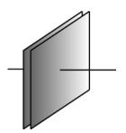
Figure 2b: Less Area – Less Capacitance
