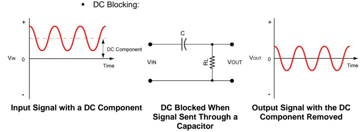
Figure 6: DC Filtering, DC is blocked and AC is passed
