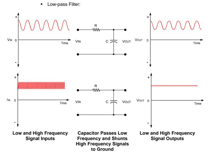
Figure 8: Capacitor in Bypass or Low-Pass Filter Configuration
