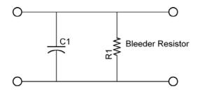
Figure 12: Bleeder Resistor across a Capacitor
