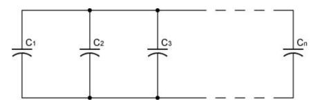
Figure 13: Parallel Capacitors
