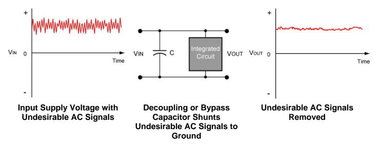
Figure 7: Undesirable AC Ripple Removed through a Decoupling Capacitor
