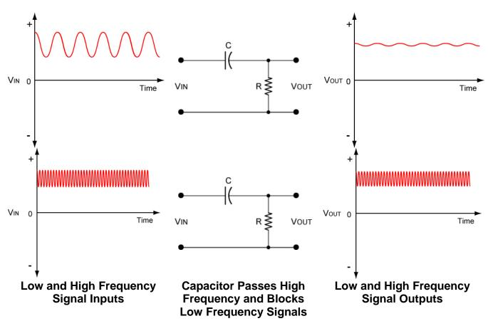
Figure 9: Capacitor in Coupling or High-Pass Filter Configuration
