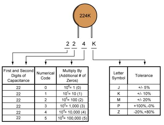
Table 2: Ceramic Disk Capacitor Standard Code (pF)
