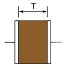
Figure 3a: Less Thickness – More Capacitance
