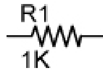
Resistor Symbol w/ Value of 1K Ohms
