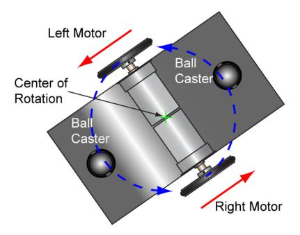
Figure 18 Turning on the Spot with Two Casters
