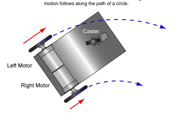
Case 3: The left motor runs faster than the right motor. The
