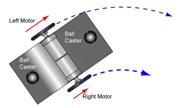
Figure 20 Arc Motion When Left Wheel Turns Faster Than the Right Wheel
