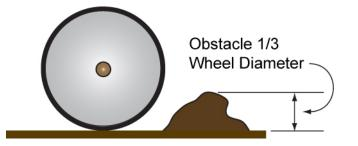
Figure 15 Typical Maximum Obstacle Height
