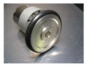
Figure 4 Solid Rubber O-ring Used as a Tire for a Wheel
