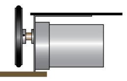
Figure 14 Side View of Improper Motor Mounting 5
