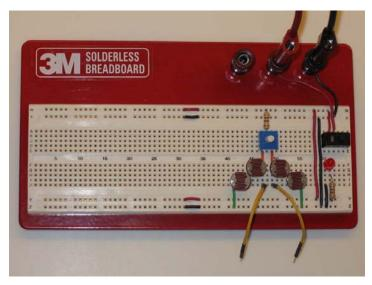
**Balanced Brightness Circuit Schematic and Layout**
