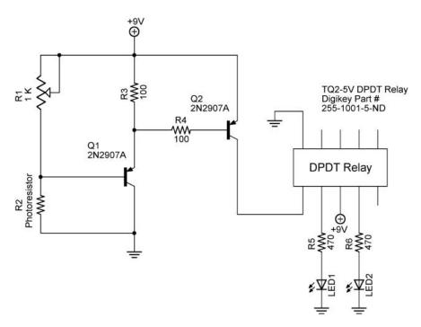
Using a photoresistor, design a light controlled circuit to vary the brightness of an LED. Wire the circuit on your breadboard and draw the schematic in the results. Remember, 9 volts applied directly to an LED will burn it out.
