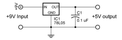
**Explanation:** A voltage regulator provides a constant dc output voltage that is nearly independent of the input voltage, output load current, and temperature. The supply voltage to a voltage regulator must be 2 - 3 volts above the regulator rating. For example, a 78L05 must have at least 7 to 8 volts as a supply to work properly. The 7800 series voltage regulators are integrated circuits (IC) that provide a positive voltage output. The 7900 series supplies a negative voltage output.
