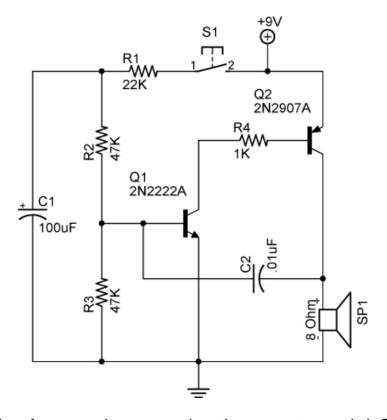
**Explanation:** Siren frequency increases when the momentary switch S1 is closed (charging the capacitor C1) and decreases when it is opened (discharging C1).
