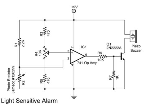
**Explanation:** The circuit uses the 741 op amp as a voltage comparator. The potentiometer R4 adjusts the light level threshold. Fine-tune R4 so the buzzer will just turn on and then block the light with your hand. The buzzer should turn off when the hand is blocking the light.
