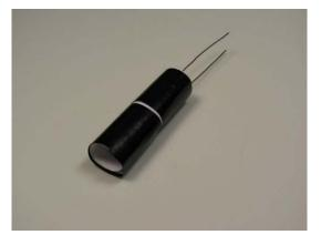
Photoresistor Inserted into Tube
