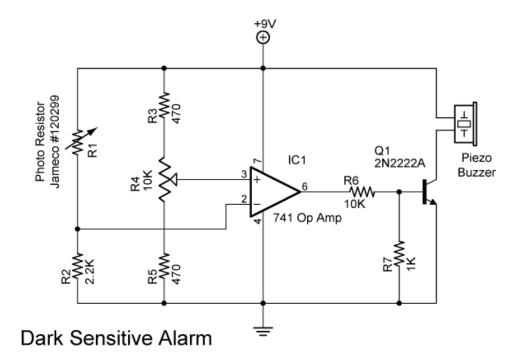
**Explanation:** By switching the R1 and R2, the circuit will become sensitive to darkness, that is, the buzzer will sound when light is blocked from the photoresistor. Adjust R4 for light levels. Adding a paper tube around the photoresistor and pointing it at a light source creates an entry alarm. See photos below.
