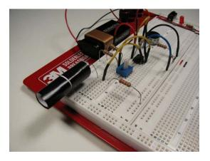
Photoresistor Pointed at Light Source
