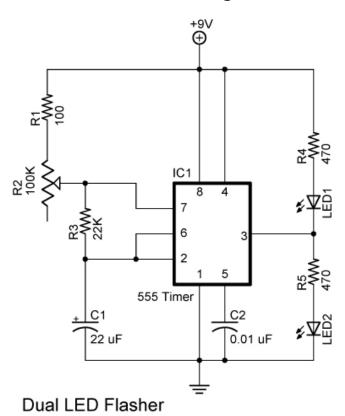
**Explanation:** R1, R2, R3, C1, and the supply voltage determine the flash rate. The lower the value of R1, R2, R3, and C1, the faster the flash rate. The *duty cycle* of the circuit (the time LED 2 is on divided by the period of the cycle expressed as percent) is determined by the ratio of R1 + R2 to R3.
